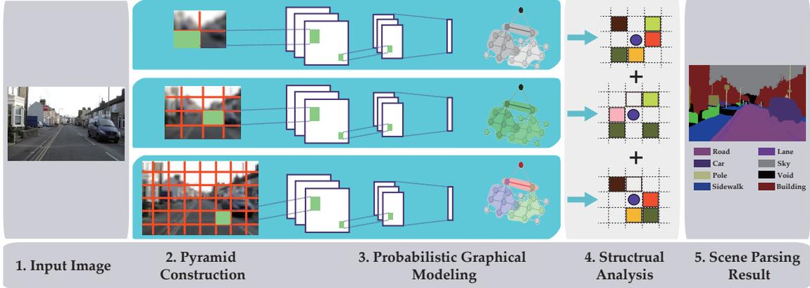
**Fig. 2.** HDPA pipeline. The input image is initially segmented under Gaussian pyramid with specific block numbers and each block is represented through a convolutional neural network. Subsequently, a probabilistic graphical model is utilized under each pyramid scale and the final pixel labels are obtained by structural analysis.
